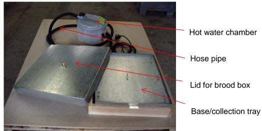
Figure 5, Steam cleaning apparatus.
