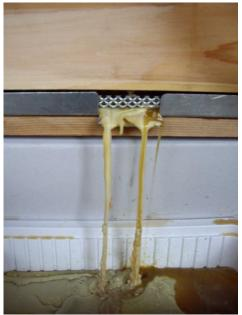
Figure 7, hot wax collecting from a steam wax extractor.
